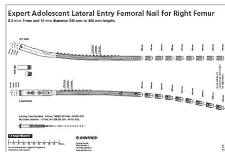
**Figure 7 (B):** The helical form of the nail and the different length.
